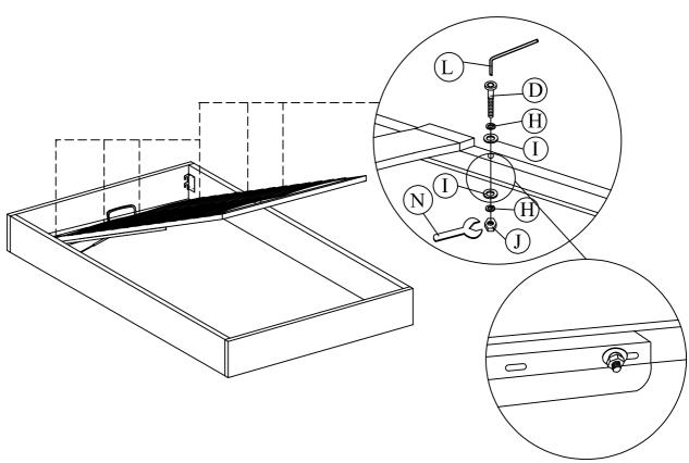
Caution: Adjust the screw at the position of the long hole as shown, then tighten the screw!
